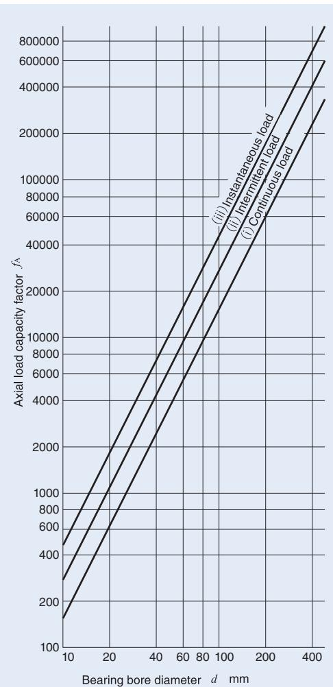
Fig. 1 Axial load capacity factor
